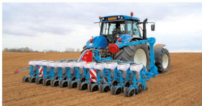
Semoir 12 rangs repliable Double-barre (45 cm d'inter-rangs)
