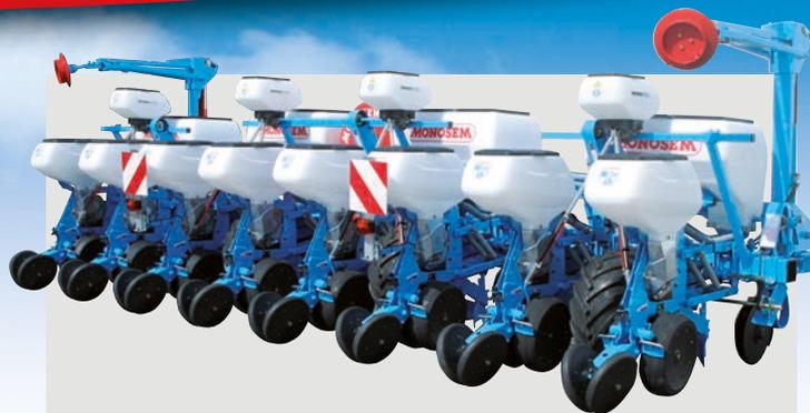
Semoir 8 rangs repliable Double-barre (75 cm d'inter-rangs)
