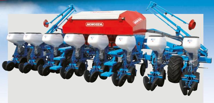
Semoir 8 rangs repliable TFC flottant (75 cm d'inter-rangs)
