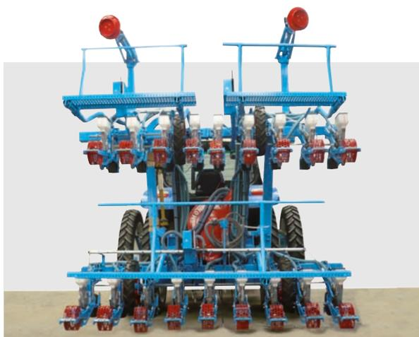
Semoir MS A - Repliable Double-barre - 18 rangs endives
